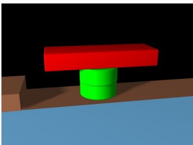
This lintel is not valid since it does not comply with rule 3 : it is not **directly** supported by 2 valid items, since the bottom most column element is not in direct contact with it.
