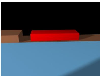
This lintel is not valid, although fully inside the construction area since it does not comply with rule 3 : it is not supported by 2 items
