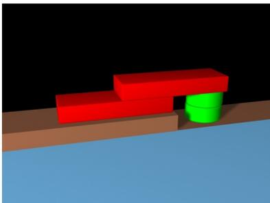
The leftmost lintel is not valid since lying directly on the construction area surface.
